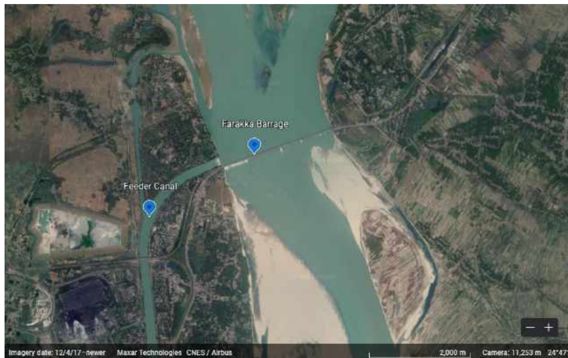
Satellite Image Showing The Divergence Of 1150 Cumecs Of Water Through The Right Bank Feeder Canal To Bhagirathi-Hooghly River, Reducing The Velocity, Pinching The Width Of The River, Causing The Emergence Of River Islands And Sluggish Flows In The Downstream Region Beyond Farakka Barrage (Google Earth, n.d.)
