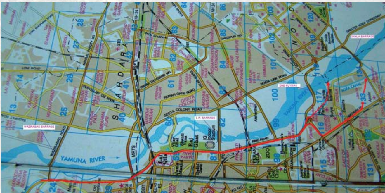
Map showing suggested alignment (red line) of a canal parallel to river Yamuna in the west bank, NCT, Delhi
